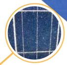
Temperature cycles can cause solder bond failures and cracks in solar cells.
