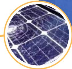
Broken glass due to corrosion.
